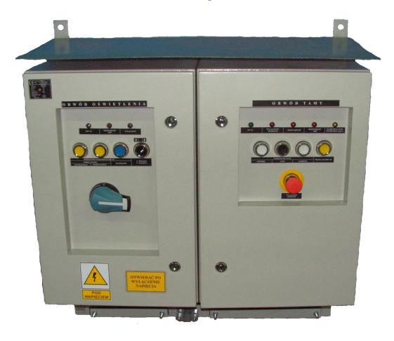
Switchgears type BTW-05/1 and BTW-05/2 are an electrical devices designed for use in underground mining in non-explosive hazard conditions as well as on the ground. Switchgears type BTW-05/1 and BTW-05/2 are designed to connecting and switching on air regulating damper, controlling the flow of air through gangways, in a 3-phase mine grid with isolated star point of the transformer (IT) for rated grid voltage of 500V.
